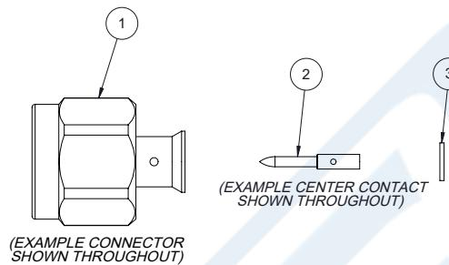
1. STRIP CABLE AS SHOWN, CHAMFER CENTER CONDUCTOR AND DEBUR CABLE.
