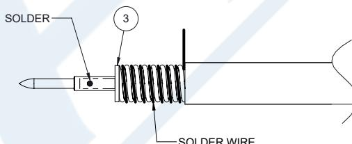
3. PUSH THE CONNECTOR BODY INTO THE CABLE, UNTIL IT STOPS. SOLDER THE CONNECTOR BODY WITH CABLE AND COVER HEATSHRINK SLEEVE.
