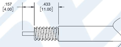
2. SLIDE INSULATOR (3) OVER CABLE CENTER CONDUCTOR. INSERT CENTER CONTACT AND SOLDER. WRAP THE CABLE BY SOLDER WIRE.
