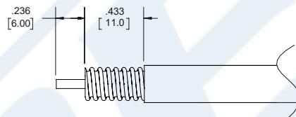
2. SLIDE INSULATOR ② OVER CABLE CENTER CONDUCTOR AND WRAP THE CABLE BY SOLDER WIRE.
