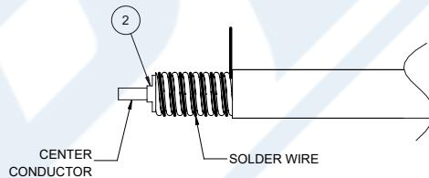
3. PUSH THE CONNECTOR BODY INTO THE CABLE, UNTIL IT STOPS. SOLDER THE CONNECTOR BODY WITH CABLE. SOLDER THE INNER CONDUCTOR. PRESS THE CAP ③ INTO BODY AND COVER HEATSHRINK SLEEVE.
