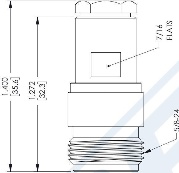
2. FORM BRAID OVER CLAMP NUT (4). SOLDER CONTACT TO CENTER CONDUCTOR. REMOVE EXCESS SOLDER. DO NOT OVER HEAT DIELECTRIC. INSERT CABLE ASSEMBLY INTO BODY & TIGHTEN.
