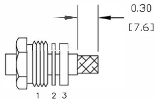
2. FORM BRAID OVER CLAMP NUT (4). TRIM BRAID BACK TO SHOULDER. CUT DIELECTRIC & CENTER CONDUCTOR TO DIMENSION SHOWN. DO NOT NICK CENTER CONDUCTOR. SOLDER CONTACT TO CENTER CONDUCTOR. REMOVE EXCESS SOLDER. DO NOT OVER HEAT DIELECTRIC. INSERT CABLE ASSEMBLY INTO BODY & TIGHTEN.
