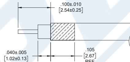
3. INSERT CENTER CONDUCTOR INTO CONTACT UNTIL DIELECTRIC BOTTOMS INSIDE CONTACT. SOFT SOLDER CONTACT TO CENTER CONDUCTOR. DO NOT OVER HEAT DIELECTRIC.
