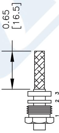
2. FORM BRAID OVER CLAMP NUT (4). TRIM BRAID FLUSH WITH SHOULDER. CUT DIELECTRIC & CENTER CONDUCTOR TO DIMENSION SHOWN. SLIDE PTFE (5) ONTO CONTACT (6), SOLDER CONTACT TO CENTER CONDUCTOR. INSERT CABLE ASSEMBLY INTO BODY & TIGHTEN.
