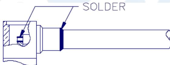
3. SOLDER CENTER CONDUCTOR TO CONTACT.
