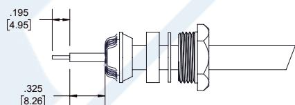
3. TIN CENTER CONDUCTOR AND SLIDE TEFLON (5) OVER INSULATOR UNTIL IT SITS AGAINST BRAID. SOLDER CONTACT (6) TO CENTER CONDUCTOR. REMOVE EXCESS SOLDER. DO NOT OVERHEAT DIELECTRIC. INSERT CABLE ASSEMBLY INTO BODY (7) & TIGHTEN.
