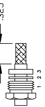
2. FORM BRAID OVER CLAMP NUT (4). TRIM BRAID BACK TO SHOULDER. CUT DIELECTRIC & CENTER CONDUCTOR TO DIMENSION SHOWN. DO NOT NICK CENTER CONDUCTOR. INSERT CABLE INTO BODY. AND TIGHTEN HARDWARE. SOLDER CENTER CONDUCTOR IN PLACE THEN & SCREW CAP DOWN.
