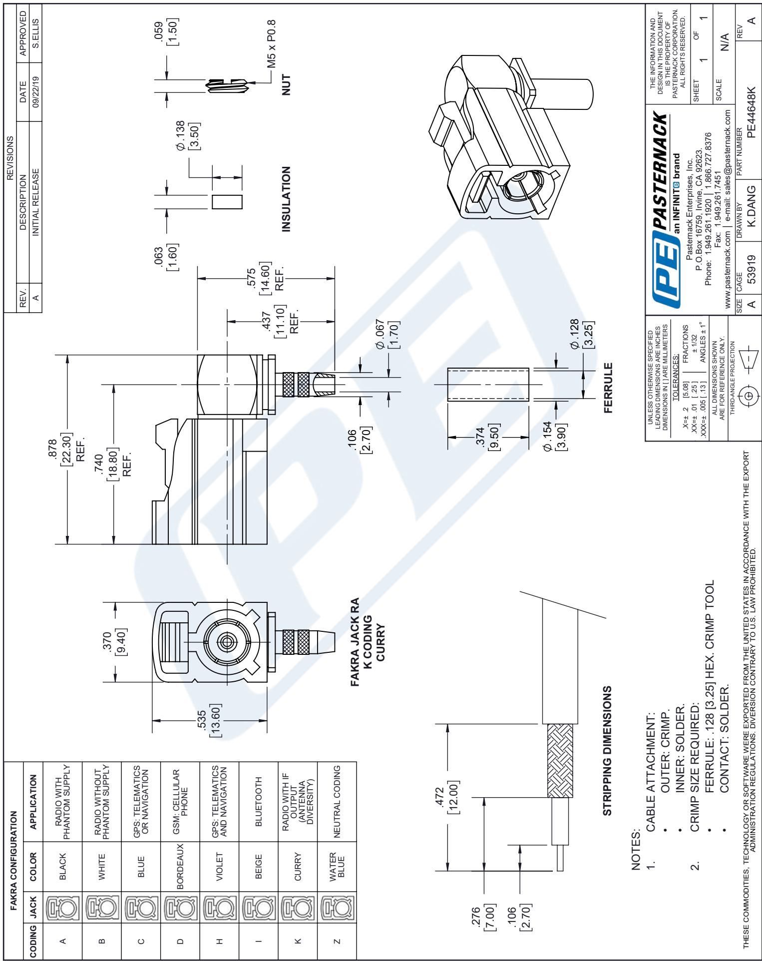
FAKRA Jack Right Angle Connector Crimp/Solder Attachment for RG174, RG316, RG188, .100 inch, PE-B100, PE-C100, LMR-100, Curry Color
