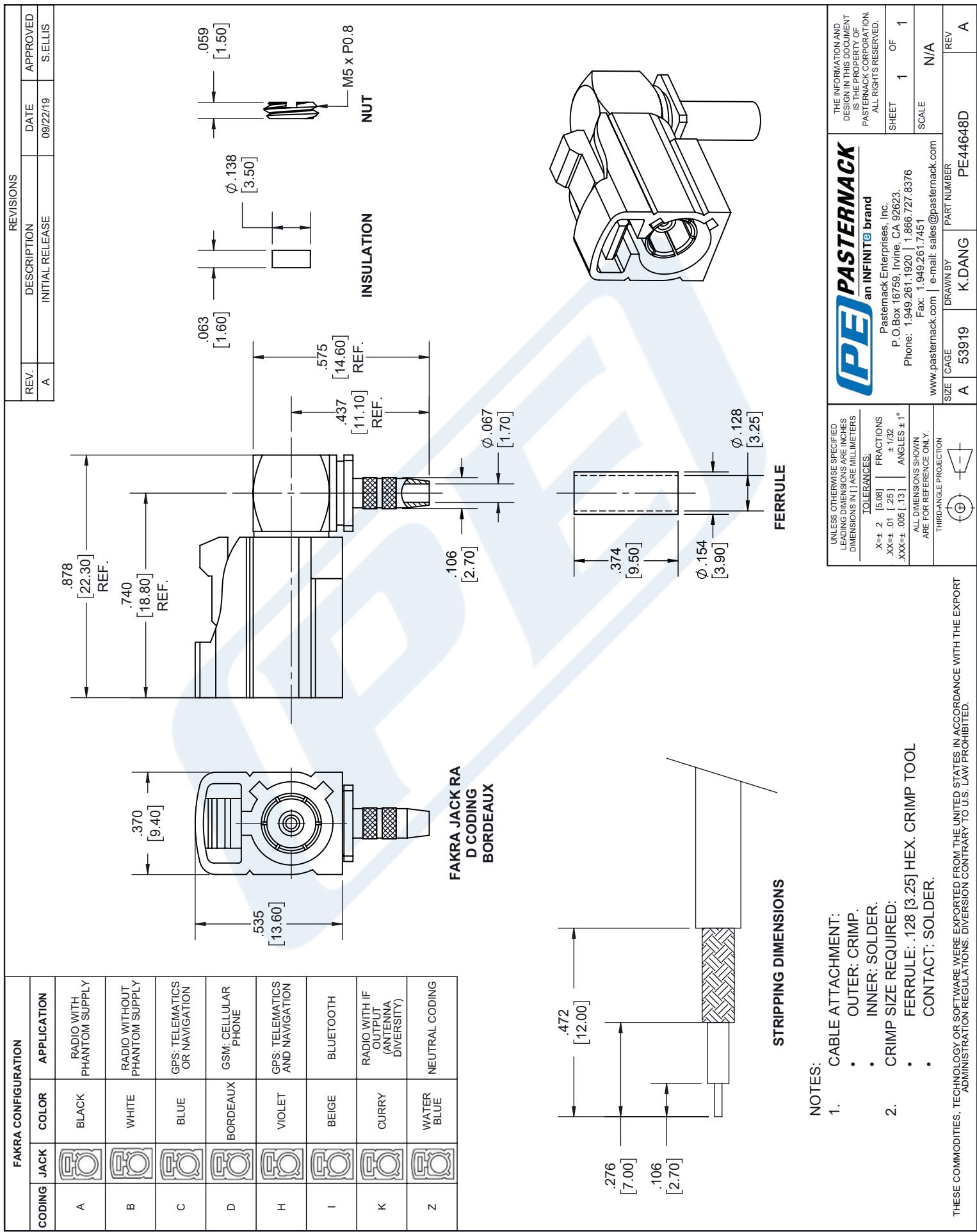
FAKRA Jack Right Angle Connector Crimp/Solder Attachment for RG174, RG316, RG188, .100 inch, PE-B100, PE-C100, LMR-100, Bordeaux Color
