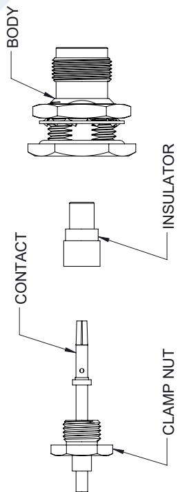
4. SOLDER OUTER CONDUCTOR TO CLAMP NUT AND TIGHTEN CLAMP NUT TO BODY.
