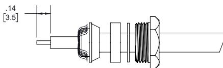
3. SOLDER CONTACT (5) TO CENTER CONDUCTOR. REMOVE EXCESS SOLDER. DO NOT OVER HEAT DIELECTRIC. INSERT ASSEMBLY INTO BODY (6) & TIGHTEN.
