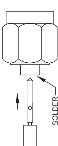
TNC Female Bulkhead Mount Connector Solder Attachment for PE-SR405AL, PE-SR405FL, PE-SR405FLJ, PE-SR405TN, RG405, IP67 Rated
