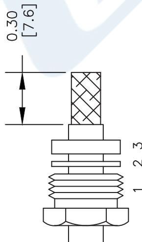
2. FORM BRAID OVER CLAMP NUT (4). TRIM BRAID BACK TO SHOULDER. CUT DIELECTRIC & CENTER CONDUCTOR TO DIMENSION SHOWN. DO NOT NICK CENTER CONDUCTOR. SOLDER CONTACT TO CENTER CONDUCTOR. REMOVE EXCESS SOLDER. DO NOT OVER HEAT DIELECTRIC. INSERT CABLE ASSEMBLY INTO BODY & TIGHTEN
