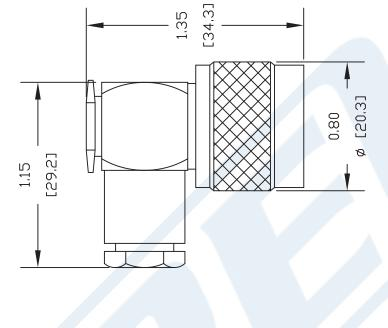
TO DIMENSION SHOWN. DO NOT NICK CENTER CONDUCTOR. TIN CENTER CONDUCTOR. SLIDE ASSEMBLY FORM BRAID OVER CLAMP NUT (4). CUT DIELECTRIC NTO BODY, SOLDER CENTER CONDUCTOR IN PLACE & TIGHTEN CLAMP NUT. SCREW CAP DOWN INTO PLACE. INTO BODY,
