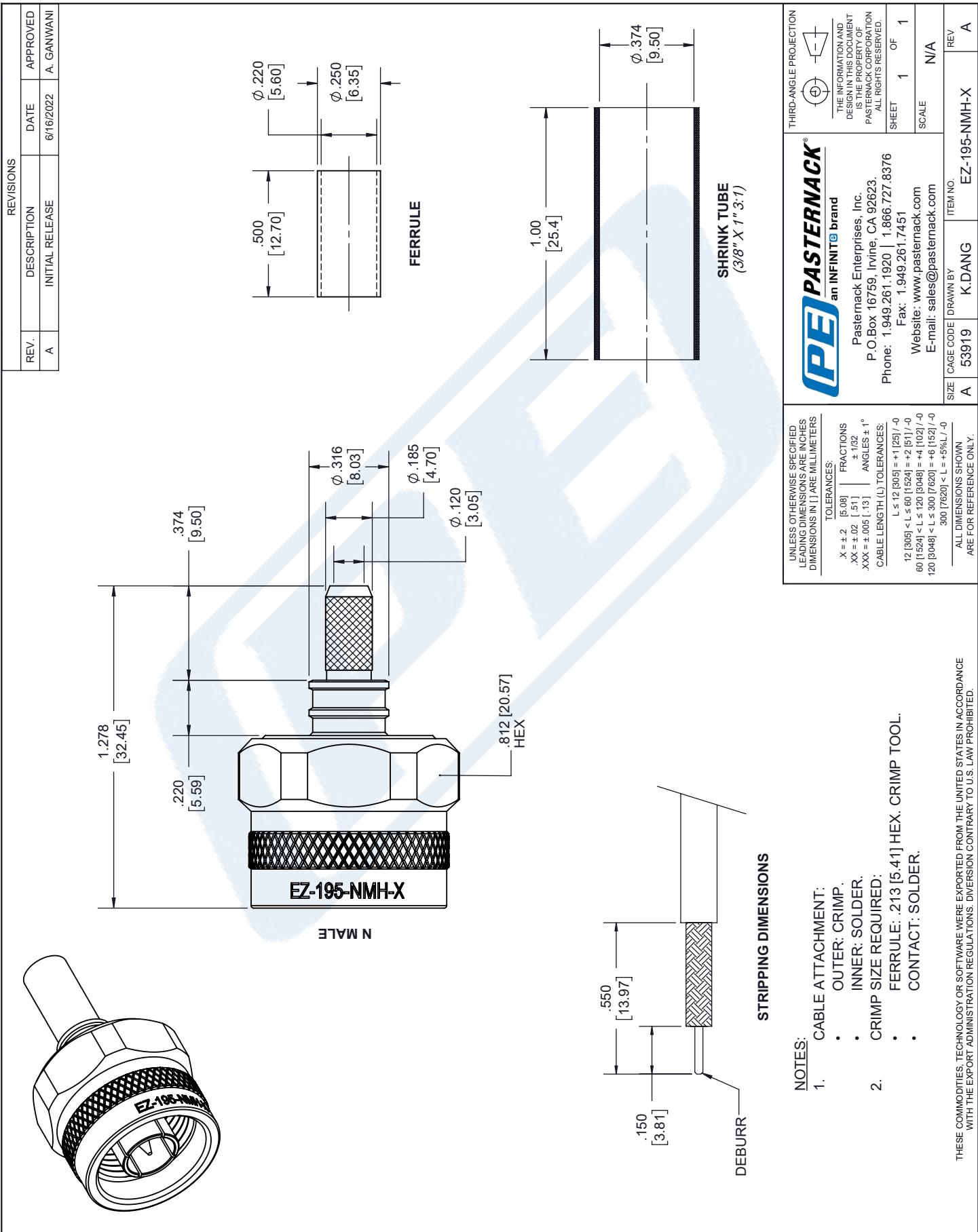
N Female Connector Clamp/Solder Attachment for
