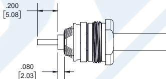
3. SLIDE WASHER (4) AGAINST THE BRAID CLAMP (3) AND HOLD BRAID IN PLACE. SLIDE HALF-INSULATOR (5) BEFORE SOLDER CONTACT (6) TO CENTER CONDUCTOR. SOLDER & REMOVE EXCESS SOLDER. DO NOT OVER HEAT DIELECTRIC. SLIDE A REST HAFT-INSULATOR (5) TO LOCKED CONTACT. INSERT CABLE ASSEMBLY INTO BODY (7) & TIGHTEN.
