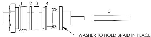
4. INSTALL CONTACT (5) BY SOLDERING TO CABLE CENTER CONDUCTOR LEAVING NO GAPS.
