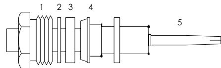
5. REMOVE EXCESS SOLDER, INSERT ASSEMBLY INTO CONNECTOR BODY AND TIGHTEN NUT TO 21 IN LBS.
