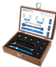
3.5mm SOLT VNA Calibration Kit Operating from DC to 26.5 GHz, Including Short Circuit, Open Circuit, Load, and Thru
