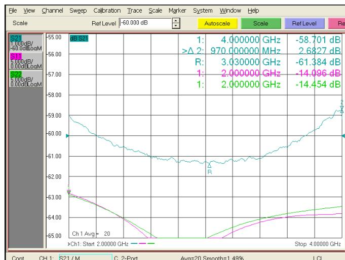
Voltage Variable PIN Diode Attenuator, 0 to 60 dB, 2 GHz to 4 GHz, SMA, 15-Pin D-Subminiature Control
