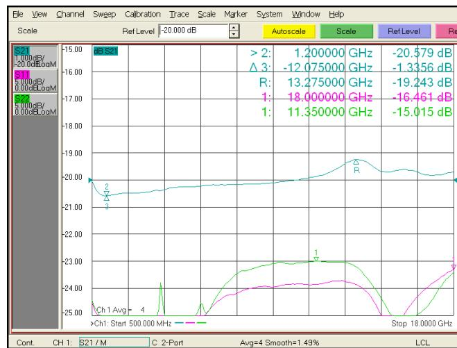
60 dB With 10 Bit Programmable TTL Controlled Attenuator, SMA Female To SMA Female, 0.06 dB Steps From 500 MHz To 18 GHz
