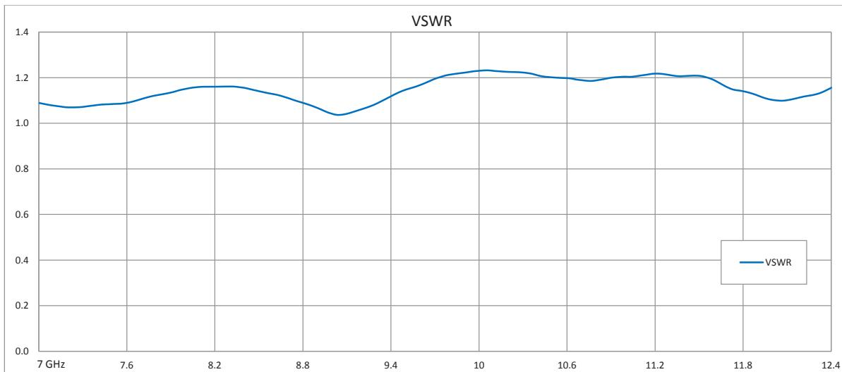
High Power Circulator With 20 dB Isolation From 7 GHz to 12.4 GHz, 50 Watts And N Female
