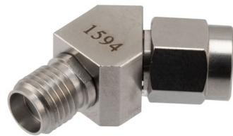
RF Adapter, 45 Degree Angle SMA plug to SMA jack 27GHz VSWR1.15
