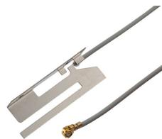
2400-2500/ 5150-5825 MHz, 4.8/3.7 dBi, Stamped Metal AP/Router Embedded Antenna With IPEX Connector
