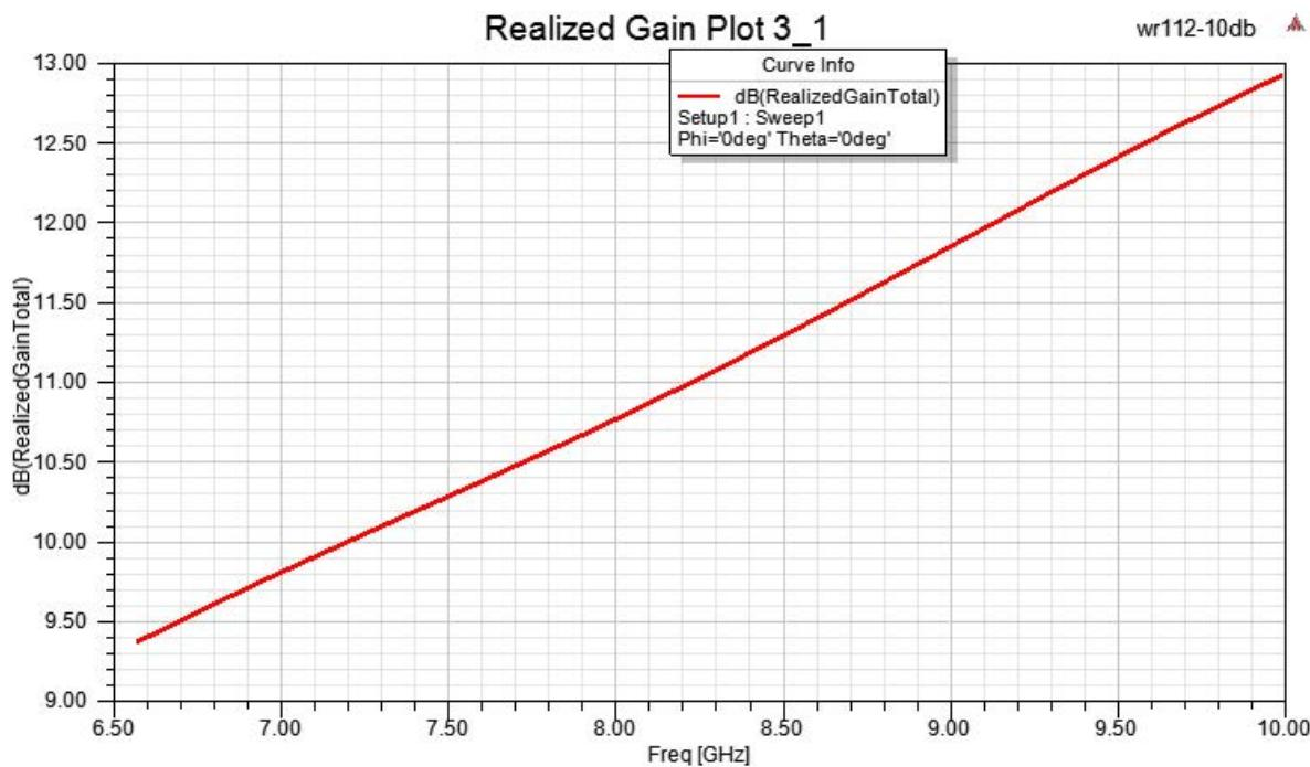
WR-112 Standard Gain Horn with 10 dBi
