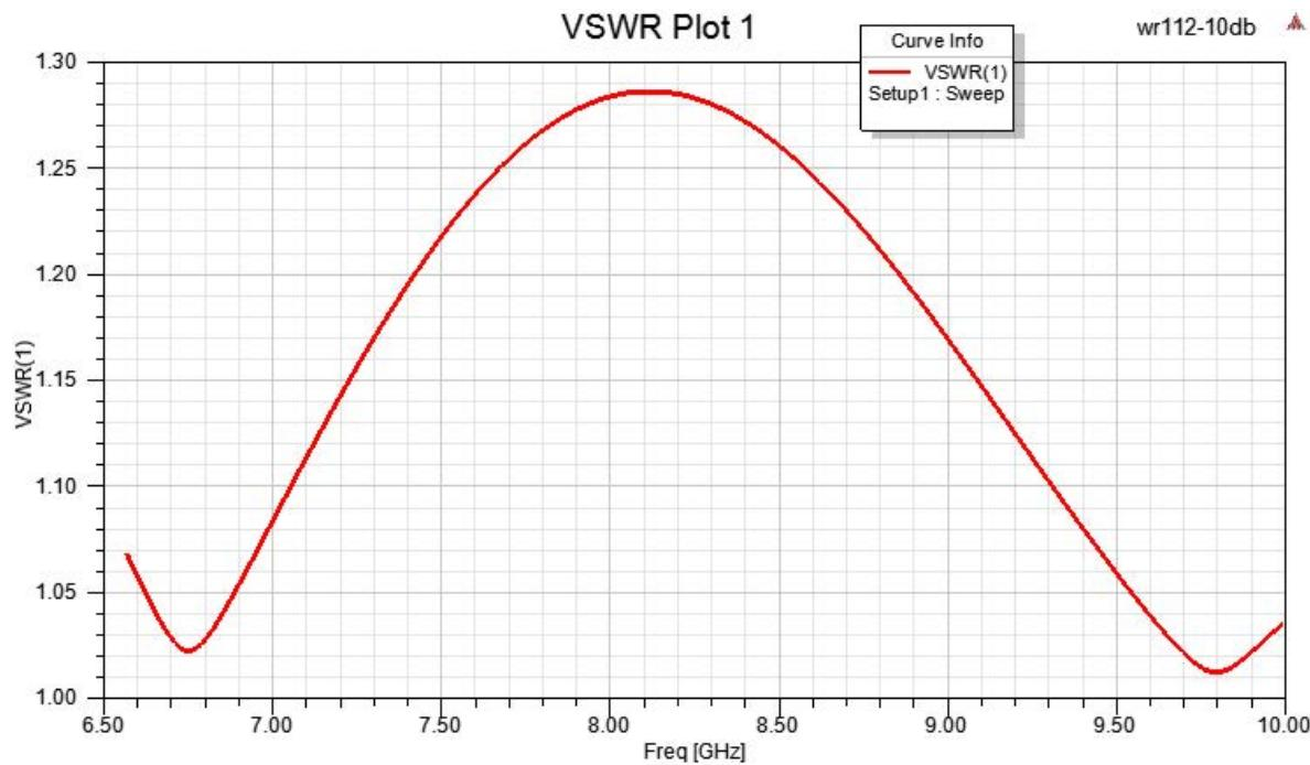
WR-112 Standard Gain Horn with 10 dBi
