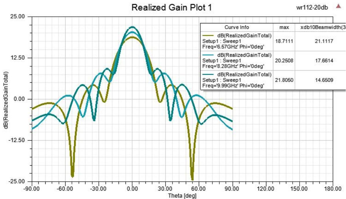
WR-112 Standard Gain Horn with 20 dBi
