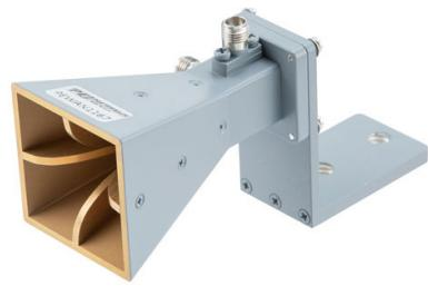
Broadband Horn Antenna, Dual Polarized 18 GHz to 40 GHz 15 dBi Gain, 2.92mm Female Connector from Pasternack Enterprises has same day shipment for domestic and International orders. Our RF, microwave and millimeter wave products maintain a 99.4% availability and are part of the broadest selection in the industry.
