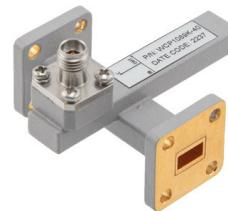
WR-28 Waveguide 40 dB Crossguide Coupler, UG Cover Flange, 2.92mm Female Coupled Port, 26.5 GHz to 40 GHz, Brass
