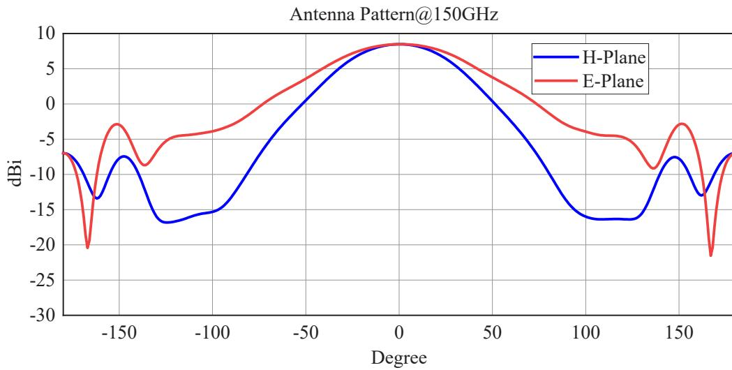
WR-6 Waveguide Probe Antenna Operating from 110 GHz to 170 GHz, 6.5 dBi Nominal Gain, UG-387/U-M Flange
