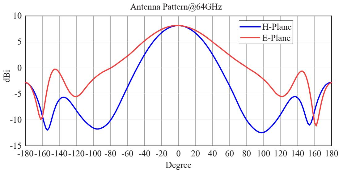
WR-15 Waveguide Probe Antenna Operating from 50 GHz to 75 GHz, 6.5 dBi Nominal Gain, UG-385/U Flange
