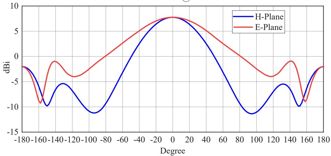
WR-22 Waveguide Probe Antenna Operating from 33 GHz to 50 GHz, 6.5 dBi Nominal Gain, UG-383/U Flange
