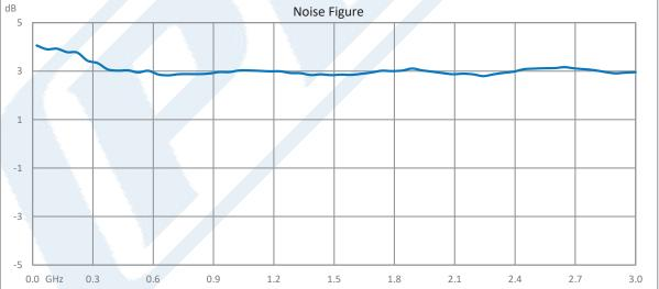
Click the following link (or enter part number in "SEARCH" on website) to obtain additional part information including price, inventory and certifications: 1 Watt P1dB, 30 MHz to 3 GHz, Medium Power GaAs Amplifier, SMA Input, SMA Output, 27 dB Gain, 39 dBm IP3 PE15A4017
